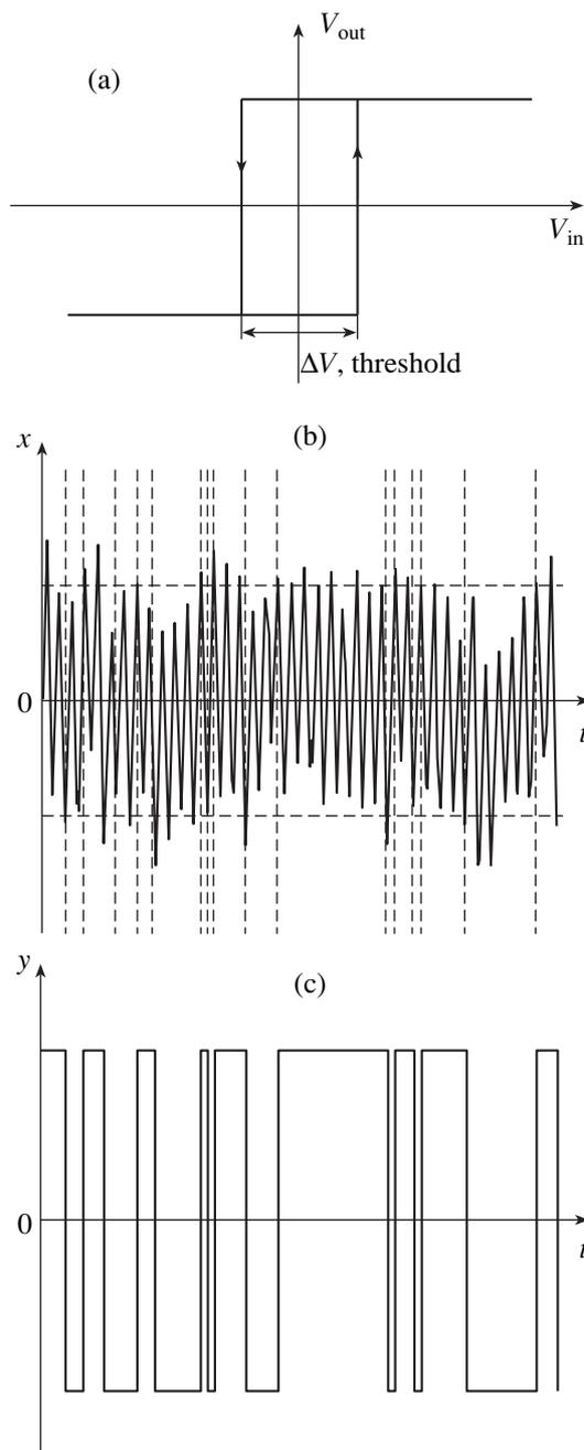
**Fig. 13.** (a) The characteristic of the Schmitt trigger; (b) the input signal  $x(t) = s(t) + \eta(t)$  of the Schmitt trigger, where  $s(t) = 0.25 \sin(0.1t)$  and  $\eta(t)$  is colored noise with a correlation time of  $\tau_c = 0.1$ ; and (c) the output signal  $y(t)$ . The dashed lines indicate the switching moments of the trigger.
