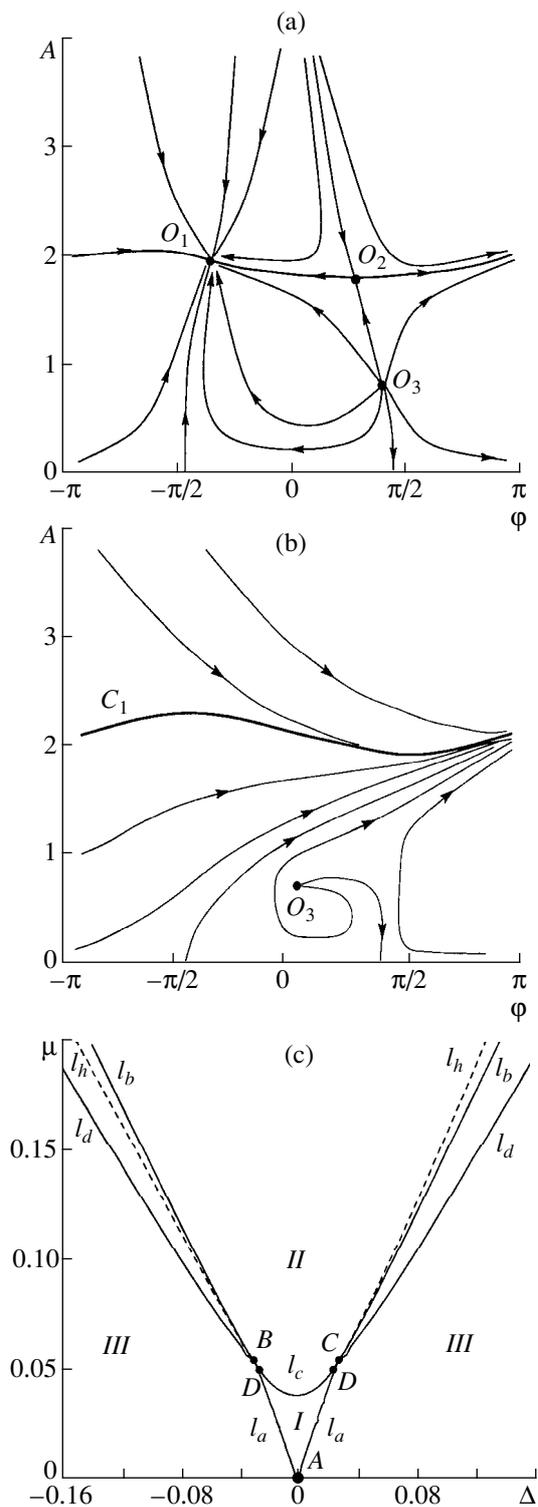
**Fig. 1.** Phase portraits of system (4) with  $\epsilon = 0$ , and  $\mu = 0.052$  for (a)  $\Delta = 0.026$  and (b)  $\Delta = 0.032$ ; (c) bifurcation lines of systems (4) and (1) on the plane of parameters  $\Delta$  and  $\mu$ .
