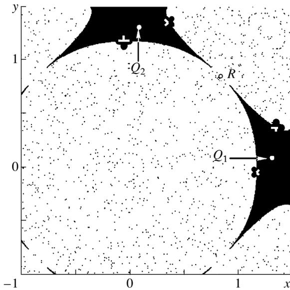
**Fig. 8.** Bistability and riddling in a system of coupled logistic maps (41) for  $r = 1.56$  and  $\gamma = 0.143$ . In addition to a chaotic in-phase attractor situated on the bisector  $x = y$ , there exists an out-of-phase stable cycle of period 2 (it contains the points  $Q_{1,2}$ ). The attraction basin of the out-of-phase attractor is marked by dark dots.
