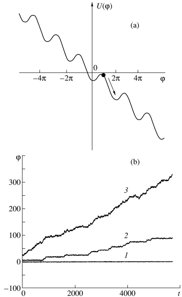
**Fig. 4.** (a) Periodic potential function  $U(\varphi)$  for Eq. (9) and (b) function  $\varphi(t)$  for various values of noise intensity  $D$ : (1)  $D = 0.02$ , (2)  $D = 0.07$ , and (3)  $D = 0.22$ ;  $\Delta = 0.06$  and  $\varepsilon = 0.15$ .
