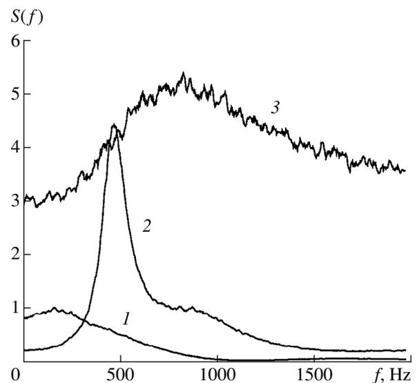
**Fig. 18.** Typical power spectra of the output signal measured in a radiophysical experiment: (1)  $D = 15 \text{ mV}^2$ , (2)  $D = 100 \text{ mV}^2$ , and (3)  $D = 600 \text{ mV}^2$ .
