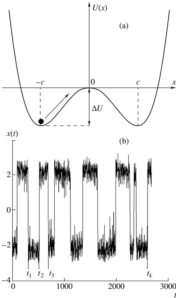
**Fig. 11.** (a) Bistable potential of system (43) and (b) realization  $x(t)$  obtained by integrating system (44).
