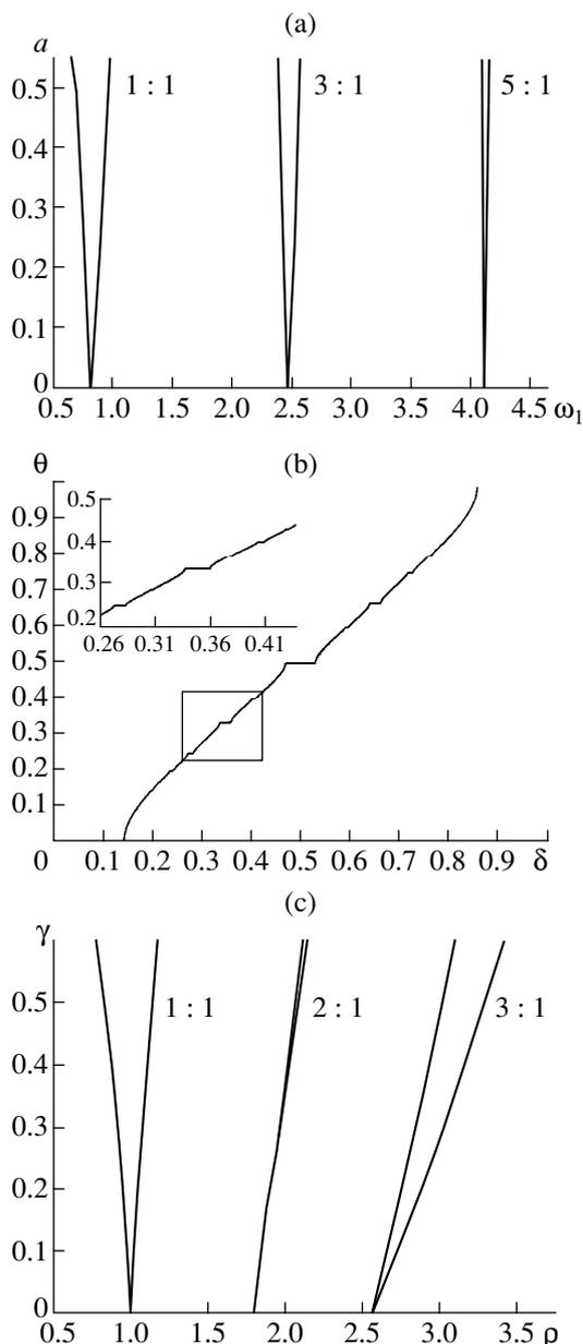
**Fig. 3.** (a) Synchronization domains of system (1) with rotation numbers of  $\theta = 1 : 1, 3 : 1,$  and  $5 : 1$ ; (b) rotation number  $\theta$  versus parameter  $\delta$  in map (5) for  $K = 0.9$ ; and (c) synchronization domains on the plane of parameters  $\gamma$  and  $p$  in system (6).
