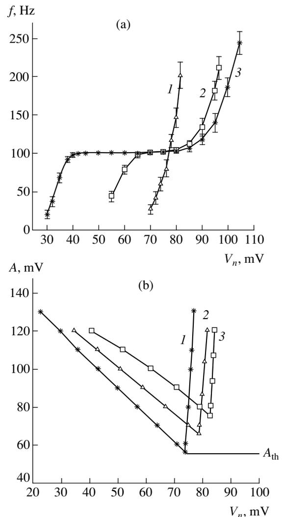
**Fig. 14.** (a) Experimental dependence of the mean frequency of the output signal of the Schmitt trigger on the noise amplitude  $V_n$  for various amplitudes  $A$  of signal: (1)  $A = 0$  mV, (2)  $A = 60$  mV, and (3)  $A = 100$  mV and (b) synchronization domains of the Schmitt trigger for various frequencies of the signal: (1)  $f_0 = 100$  Hz, (2)  $f_0 = 250$  Hz, and (3)  $f_0 = 500$  Hz.
