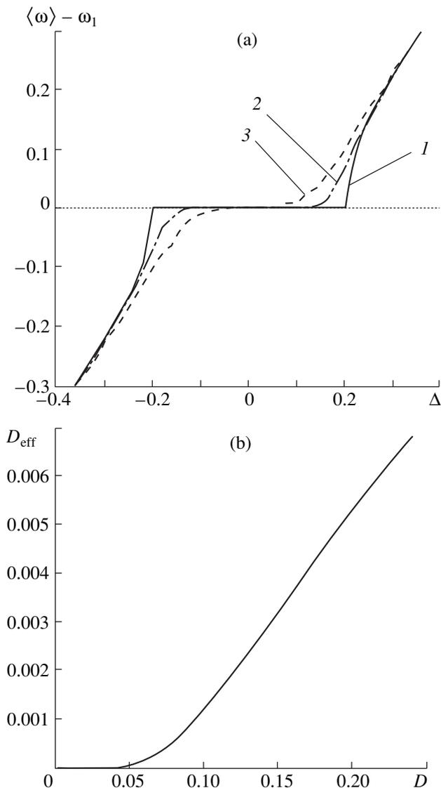
**Fig. 5.** (a) The difference between the mean oscillation frequency calculated by (9) and the driving frequency as a function of the mismatch parameter for various values of noise intensity  $D$ : (1)  $D = 0$ , (2)  $D = 0.02$ , and (3)  $D = 0.07$ ; and (b) the effective diffusion coefficient  $D_{\text{eff}}$  calculated by formula (12) as a function of noise intensity under the assumption of zero mismatch.
