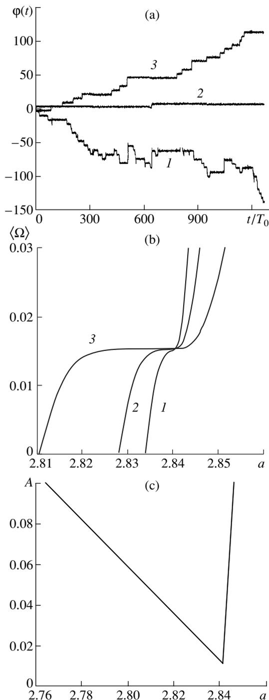
**Fig. 15.** (a) Instantaneous phase difference as a function of time for various values of the control parameter  $a$ : (1)  $a = 2.821$ , (2)  $a = 2.835$ , and (3)  $a = 2.8435$ ; (b) mean switching frequency as a function of parameter  $a$  for various signal amplitudes  $A$ : (1)  $A = 0.005$ , (2)  $A = 0.025$ , and (3)  $A = 0.01$ ; and (c) synchronization domain of switching frequency for map (54).
