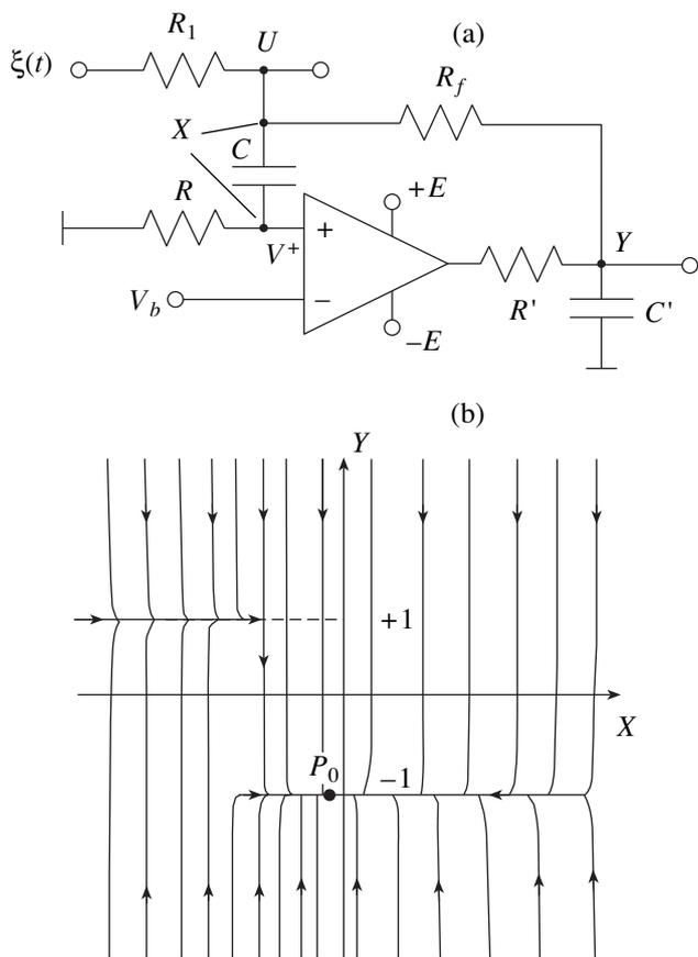
**Fig. 17.** (a) Schematic diagram of the monovibrator used in a full-scale experiment and (b) basic features of the phase portrait of system (57).
