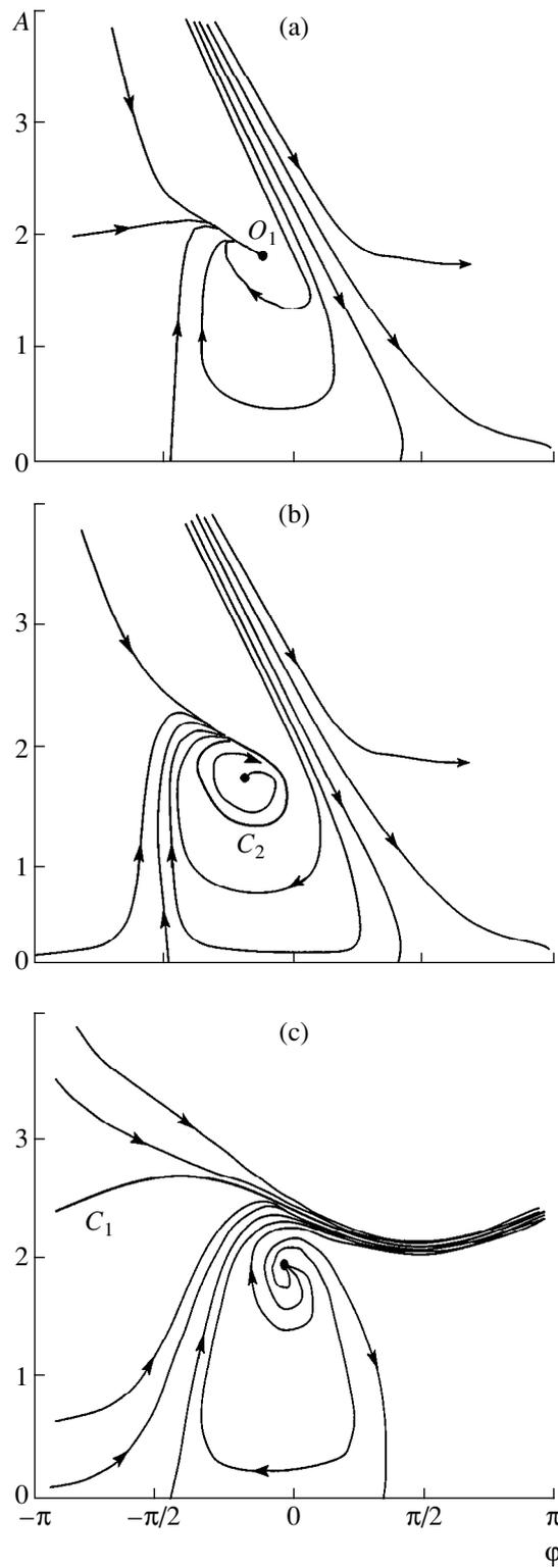
**Fig. 2.** Phase portraits of system (4) with  $\epsilon = 0$ , and  $\mu = 0.056$  for (a)  $\Delta = 0.028$ , (b)  $\Delta = 0.031$ , and (c)  $\Delta = 0.033$ .
